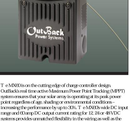
sizing of your solar array. Te ability to step-down a high voltage solar array to a low voltage battery can save you money by reducing the size of wire required and making the installation simpler and faster.
