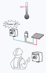
Automatic shutdown the panels when there is a temperature in the area higher than 85°C detected.
