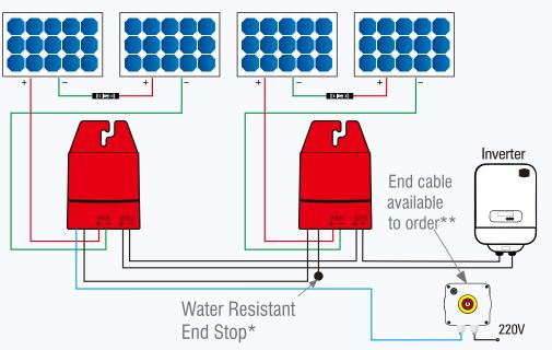
Each BFS-11 device operates two solar modules, the modules in series go to inverter string as usual. The only difference is the communication signaling cables connect the BFS-11 in series and go to the button switch complete the RSD solution.
